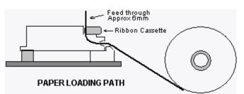
**3.** Remove old roll core from the holding fingers and insert the new roll with the paper direction as shown in the diagram above.
